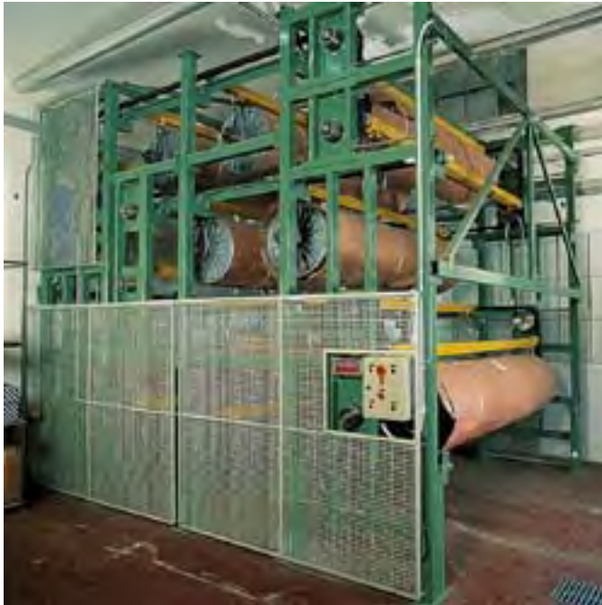
fabric rolls storage carousel system FERBER type MFR with fabric rolls suspension through chains hanging from transom in rotation
